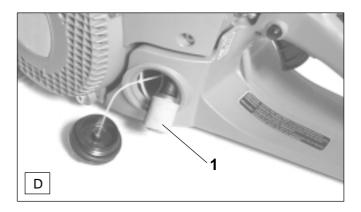
The felt filter (D/1) of the suction head can become clogged. It is recommended to replace the suction head once every three months in order to ensure unimpeded fuel flow to the carburetor.
